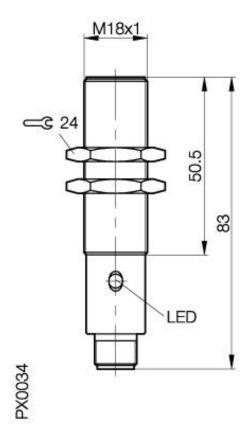
Inductive Sensors BES 515-326-S 4-C M18x1 x 83 normally-open Sn=5mm shielded
